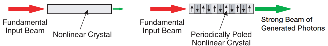
Figure 1: Comparing the generated photons of a nonlinear crystal versus a periodically poled nonlinear crystal [3]
