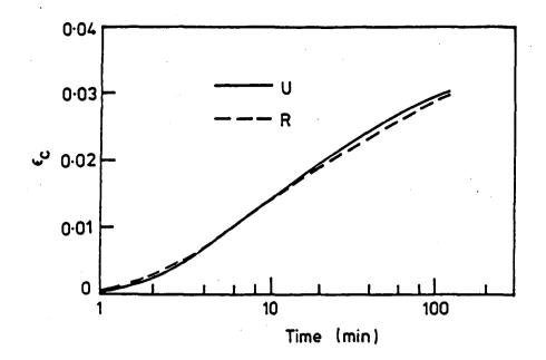
Figure 2(a). Creep strain as a function of time for unreinforced ZnO (referred to as sample U) and ZnO reinforced 10 v% SiC (sample R) sintered at 725°C under a uniaxial stress of 250 kPa.
