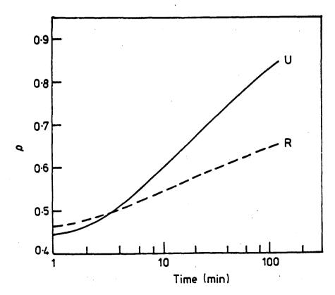
Figure 2(b). Density as function of time for samples U and R described in Fig. 2(a).
