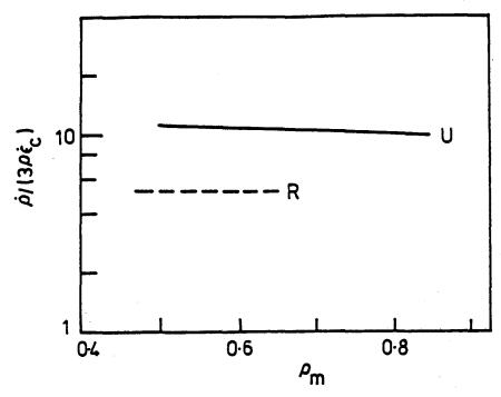
Figure 3. Ratio of the densification rate to the creep rate as a function of the matrix relative density for sampes U and R described in Fig. 2(a).
