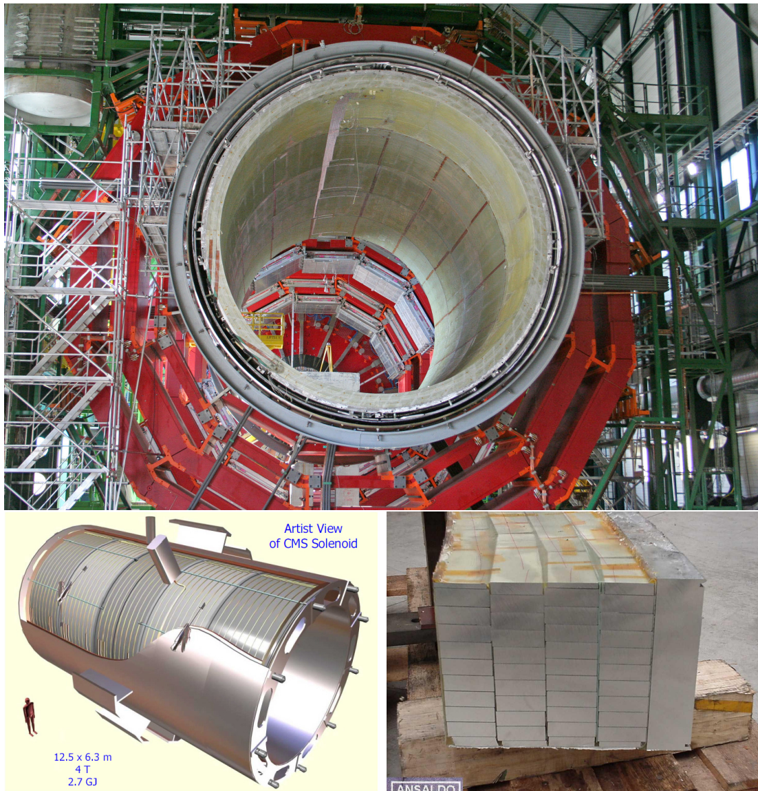
Figure 2.12: Magnet system of CMS. Colored pictures are available online [5]. The top shows the yoke(red), outer vacuum tank and the coil. The left bottom shows pictorial view of the magnet system and the right bottom shows the cross section of coils.
