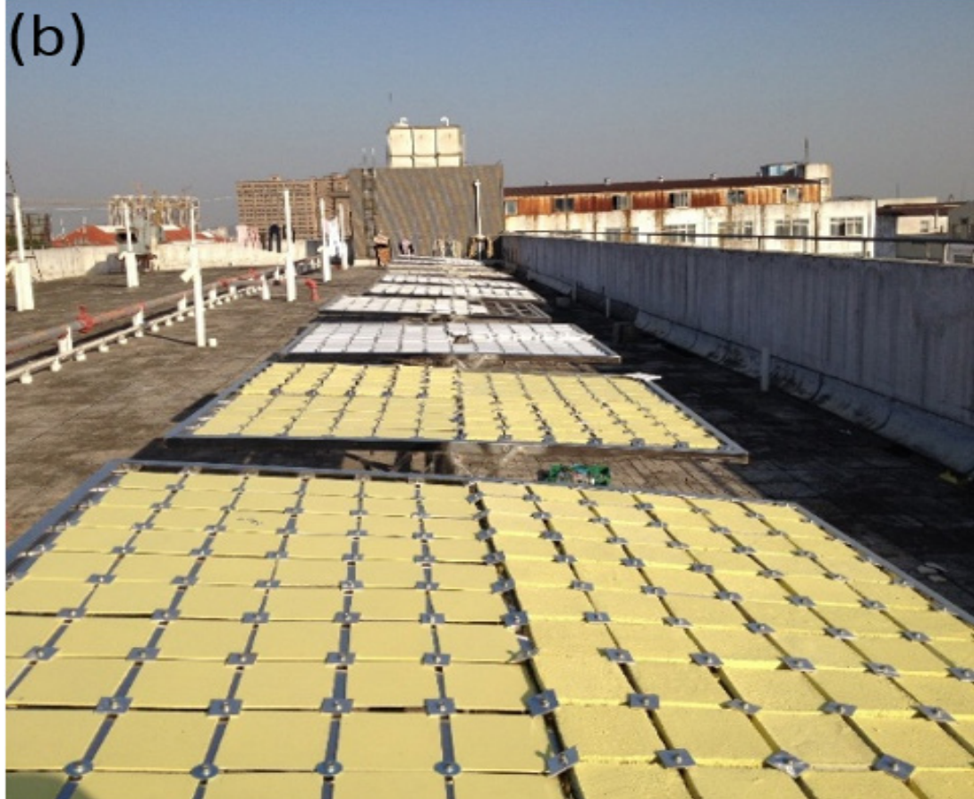
Figure 4. Natural outdoor-exposure of specimens (a) specimens location, and (b) exposure site.
