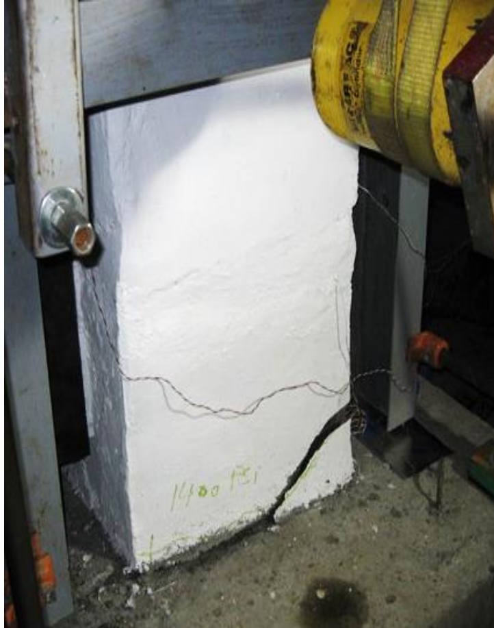
Figure (3.29): Crack Pattern for Composite I-section Column
