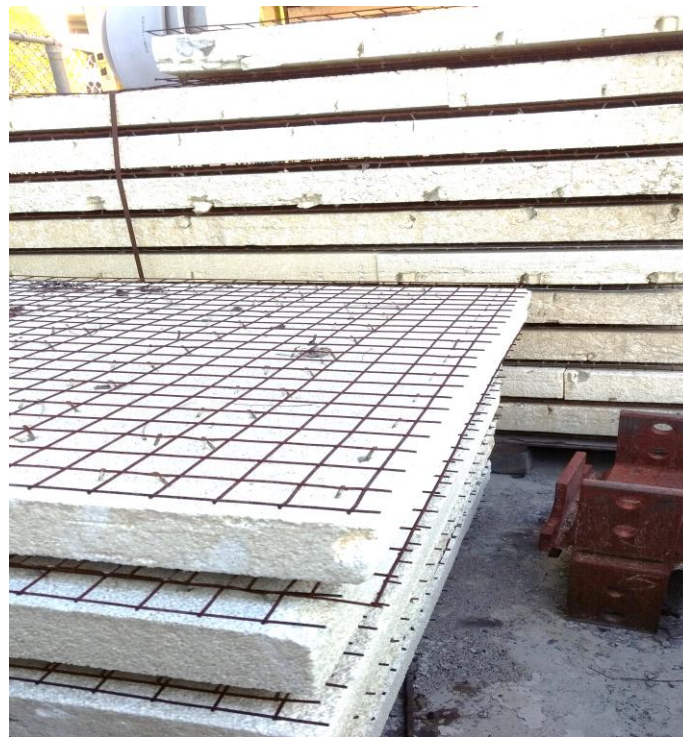
Figure (3.6): EPS Sandwich Panels with Welded-wire Reinforcements
