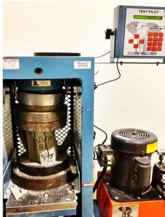
Figure (3.7): 28-day Compressive Strength Testing of Mortar Cylinder
