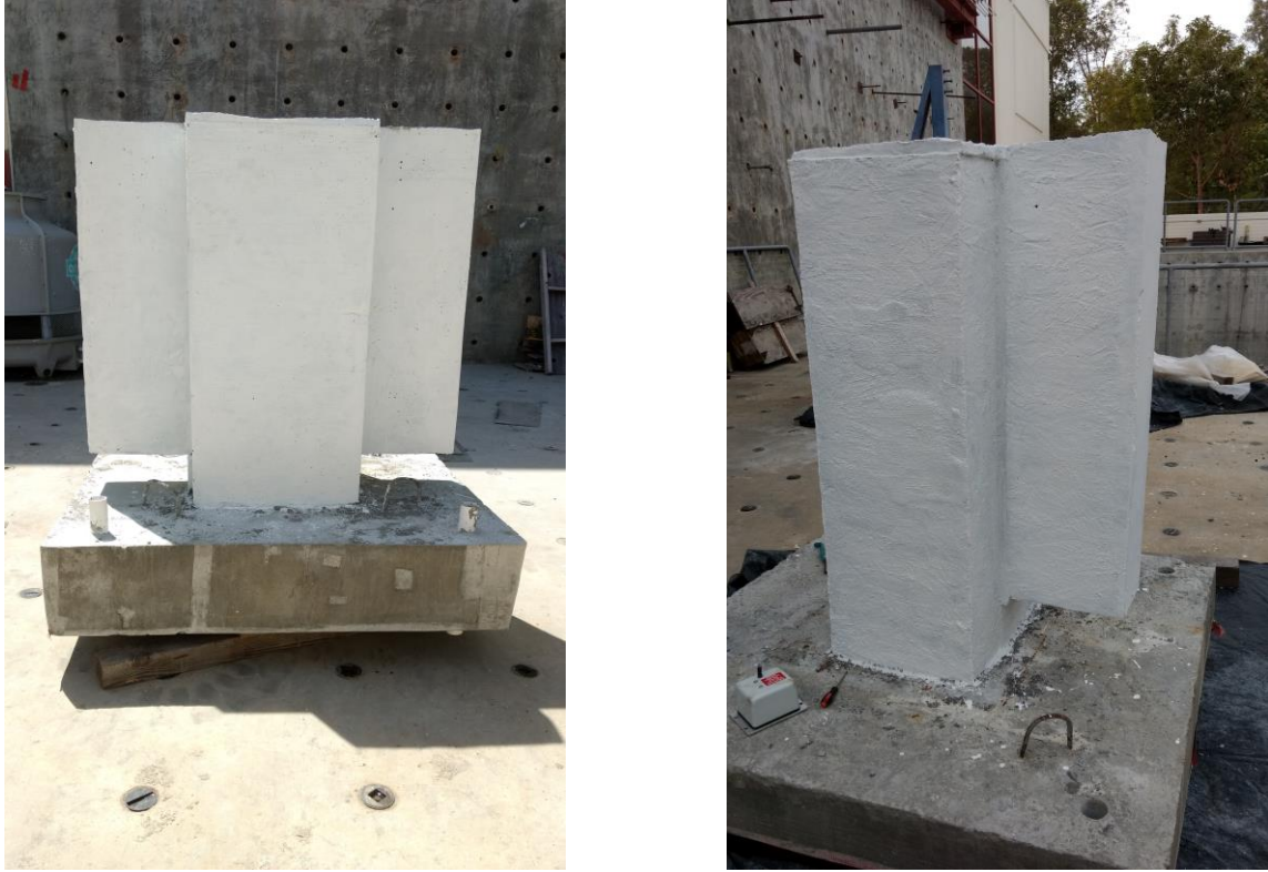
Figure (3.14): I-Section & C-Section Column Specimens After Curing & Painting
