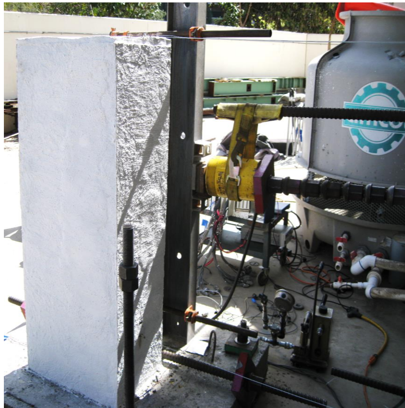
Figure (3.28): Experimental Setup for Composite C-Section
