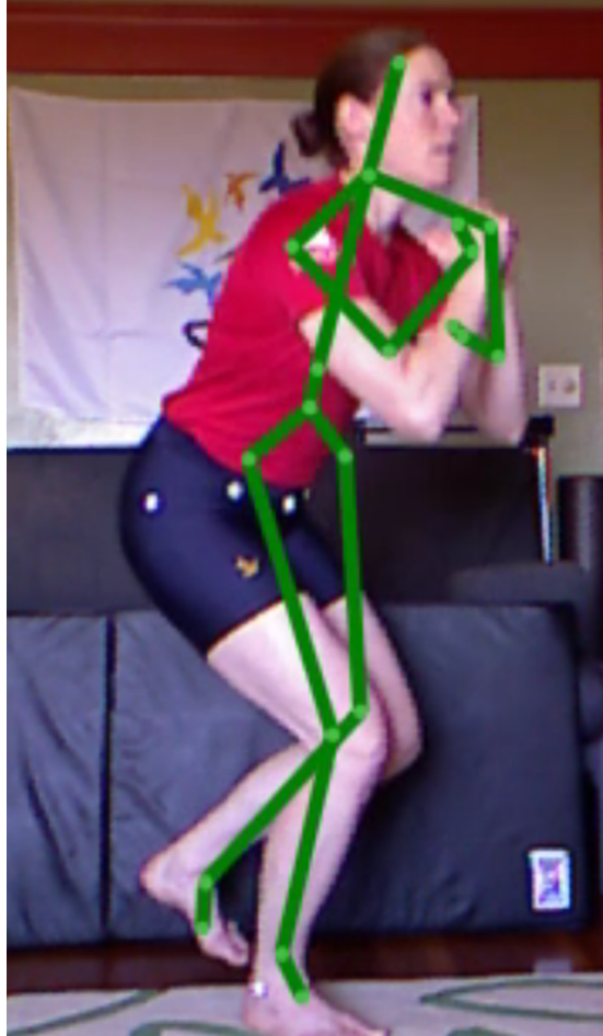
Figure 1.9: Example of 3D pose estimation (skeleton) overlaid on RGB image captured from the Microsoft Kinect during a SLS maneuver.
