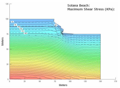
Figure 9. Theoretical shear stresses prior to the Solana Beach failure.
