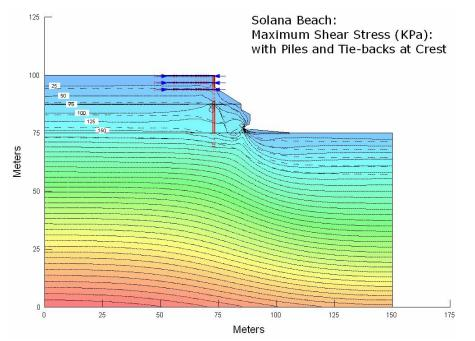
Figure 10. Theoretical stress distribution with erosion control measures.
