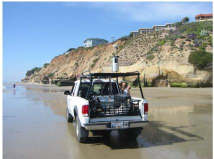
Figure 5. Mobile ground-based LIDAR setup.
