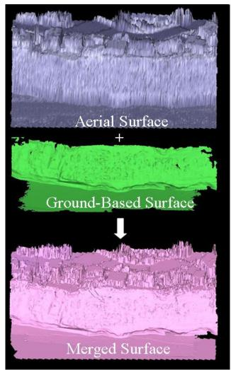
Figure 11. Merging aerial and ground-based LIDAR surfaces.
