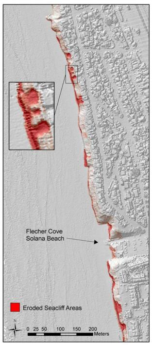
Figure 2. Areas of seacliff erosion in Solana Beach from April 1998 to April 2004.
