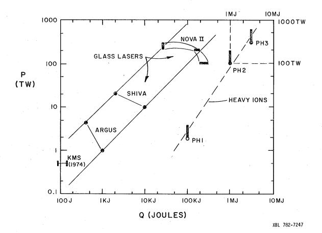
Fig. 1 - An example comparison between glass-laser systems (actual and proposed) and suggested heavy-ion phased facilities. The square (1-10) MJ, (100-1000) TW, is considered the goal for power generation. The vertical bars on the heavy-ion points indicate that the power can be increased, if wished, by doubling the number of final beams. Typically, the heavy ion driver designs have higher energy and less power than the glass laser systems.
