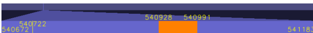
Figure 6: Control for navigation on original 1D data sequence. The upper bar corresponds to the complete sequence, and the lower bar corresponds to the displayed portion of a sequence. A highlighted region in the upper bar represents the displayed portion of the complete sequence and is connected to the lower bar, showing the correspondence of the displayed sequence portion to the complete sequence. The highlighted region in the lower bar denotes the selected octant.
