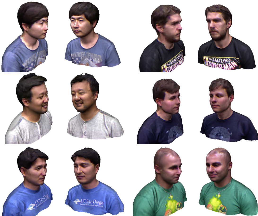
Figure 5.7: Results created with the proposed method, shown as color textured meshes. All results were computed from a handheld camera which captures depth and color images. Note that the mesh models are rendered from two view points.
