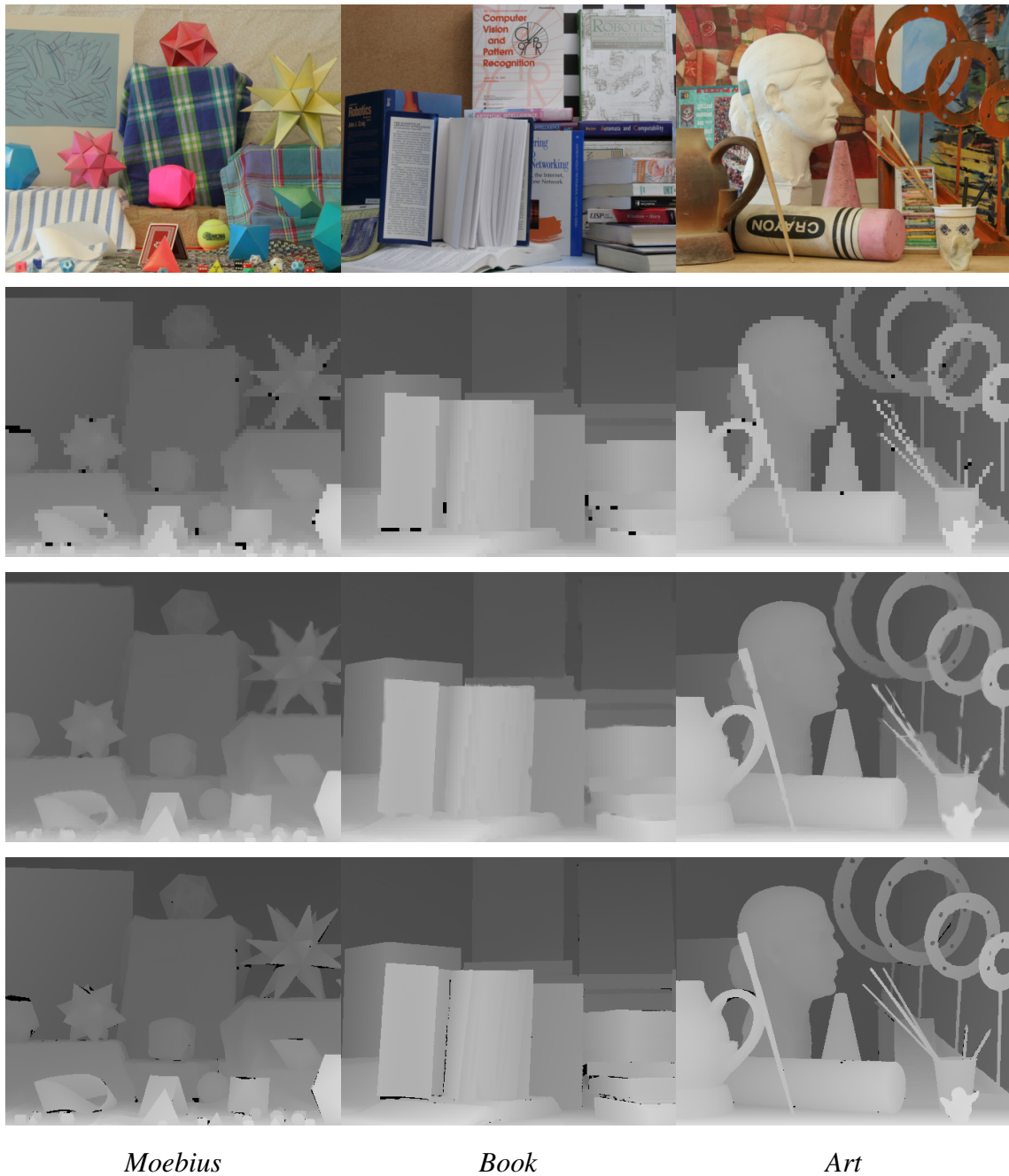
Figure 3.3: Experimental results of our method. The input disparity maps are generated by downsampling ground truth with factor of 5. (First Row) Color images, (Second Row) Input disparity map, (Third Row) Our results, and (Fourth Row) Ground truths
