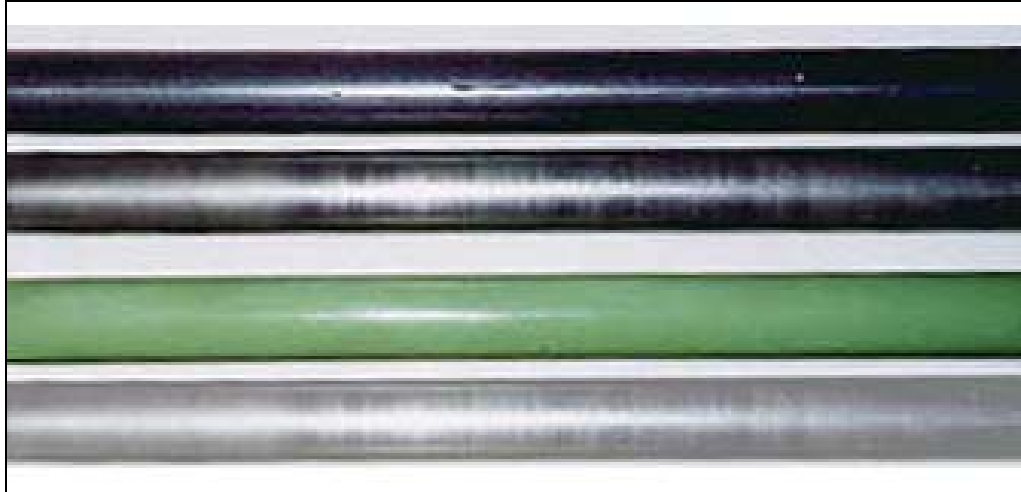
Figure 3. Steel dowel types investigated in Phase I. From top to bottom: carbon steel, stainless steel clad, carbon steel coated with bendable epoxy, and stainless steel hollow.
