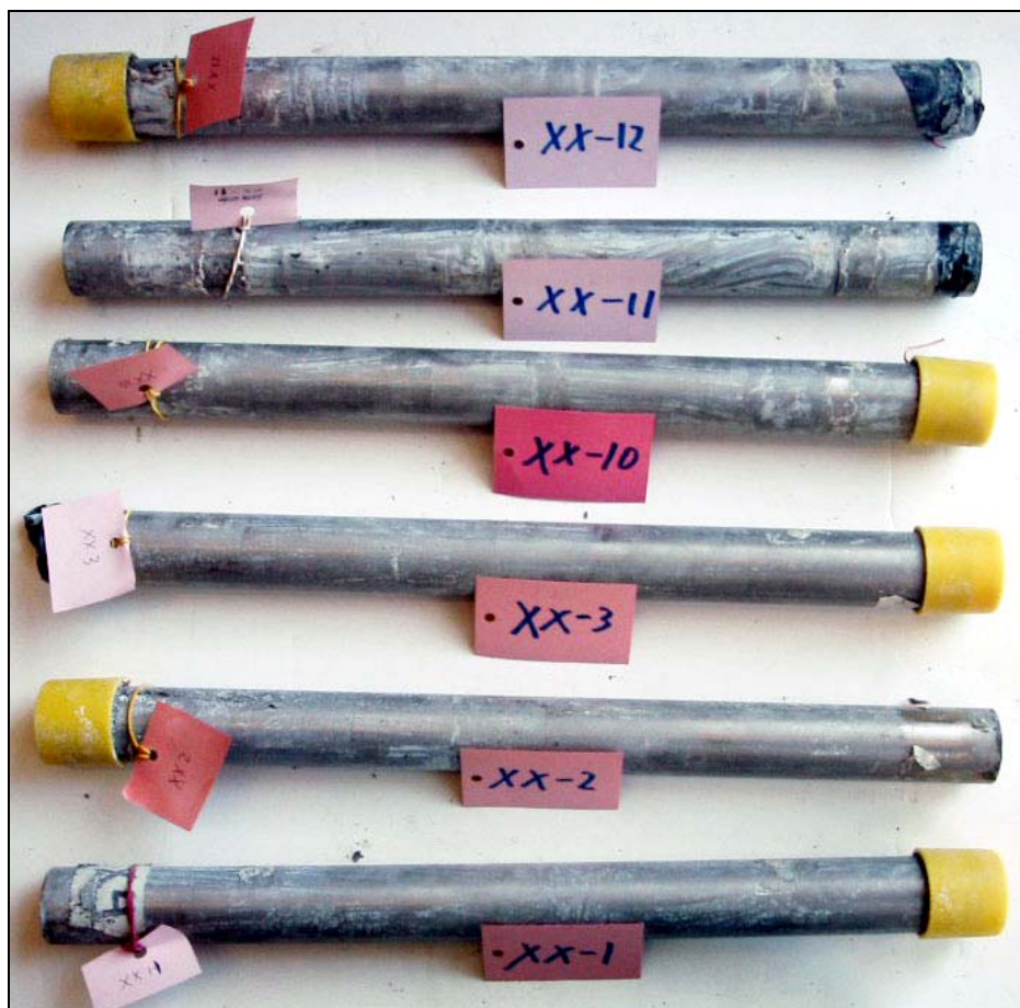
Figure 25. Appearance of stainless clad bars after tests.
