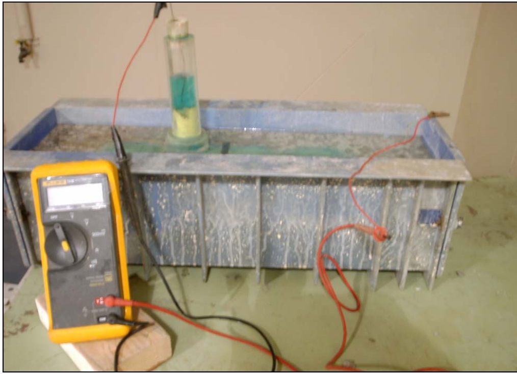
Figure 5. Half-cell potential test using a high impedance (10 Meg-Ohm) voltmeter, and a copper/copper sulfate reference cell.
