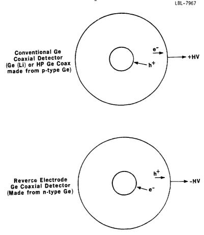
Fig. 1 Charge collection direction in germanium coaxial detectors.
