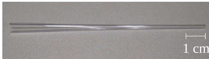
Figure 3.27: Photo of sample tapered Pyrex tube used for ion guiding experiments.
