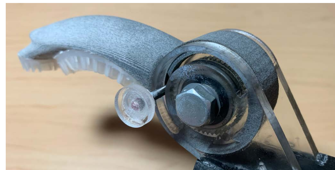
Ratchet with One-Way Bearing Assembly
