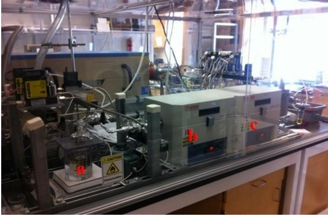
Figure 2.1: Overview of the CVD system (a) TBDS bubbler (b) Upstream furnace (c) Downstream furnace
