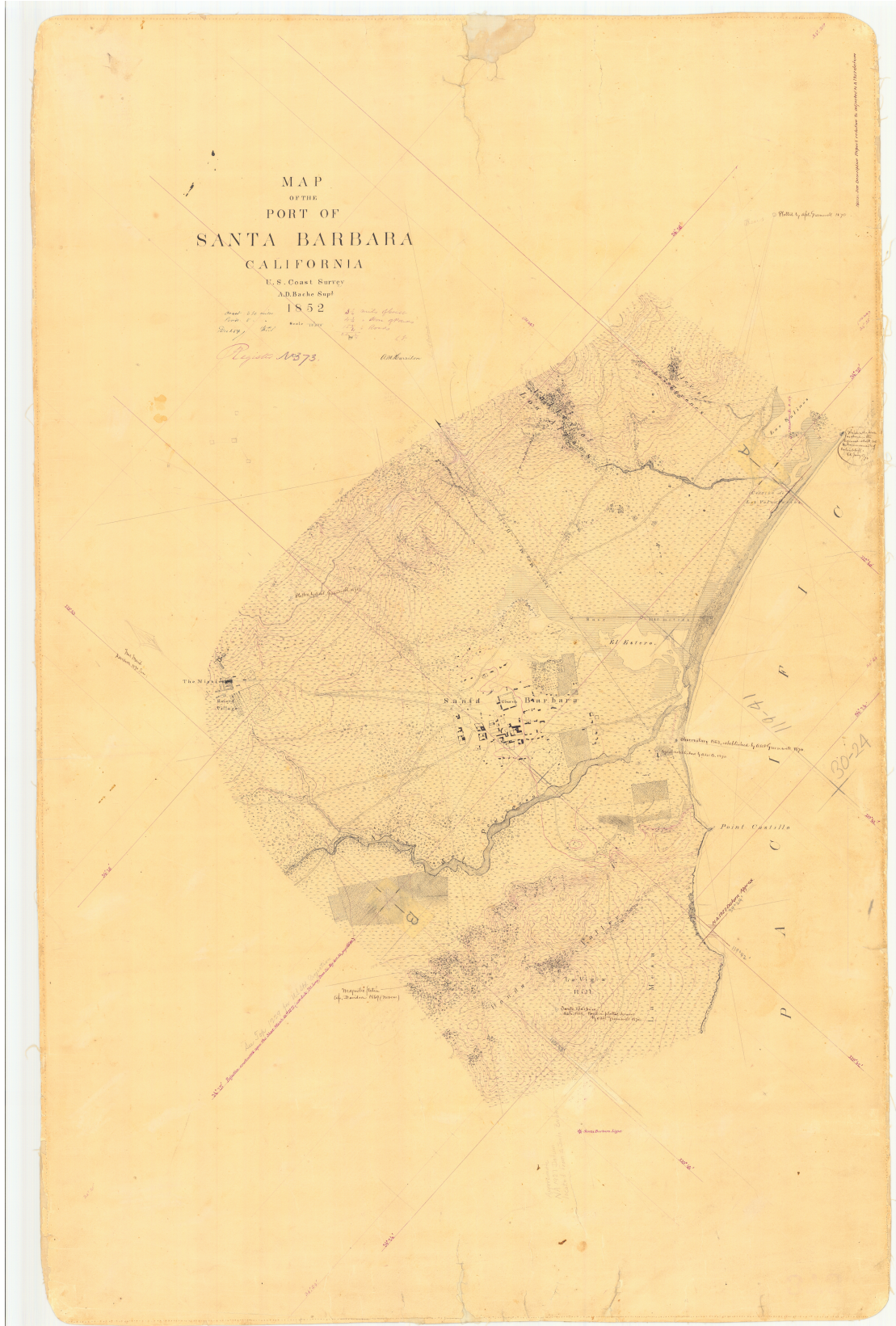
Supporting Figure 6: 1852 T-sheet of the Santa Barbara coastline detailing paleo-creek locations relative to Las Salinas Lagoon pre-modification. (San Francisco Estuary Institute)
