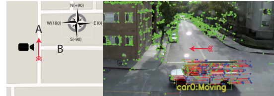
Fig. 3—Motion Analysis via Multi-Object Tracking
