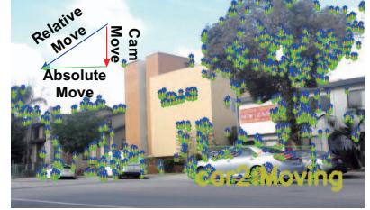
Fig. 4—Camera Movement Subtraction
