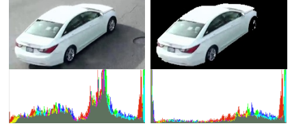
Fig. 8—Object Thumbnail and Corresponding Color Histogram Before (Left) and After (Right) Background Removal.
