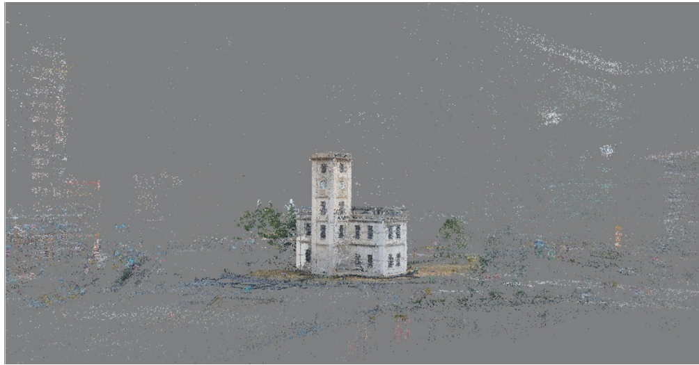
Figure 6 This picture is captured in the Agisoft Metashape, which demonstrates how the images are stitched together. Image courtesy of the author.
