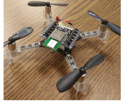
Figure 8.10: CrazyFlie 2.0 quadrotor helicopter with DW1000 UWB expansion.
