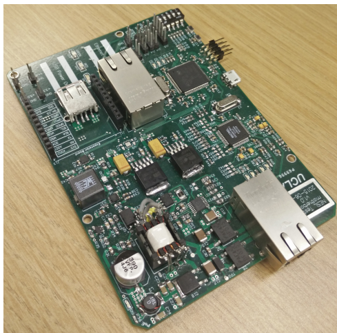
Figure 7.2: NTB Version 1.0 – power over ethernet and DUT hardware support. Figure 7.3: NTB Version 2.0 – reduced size and PTP-compliant ethernet switch.
