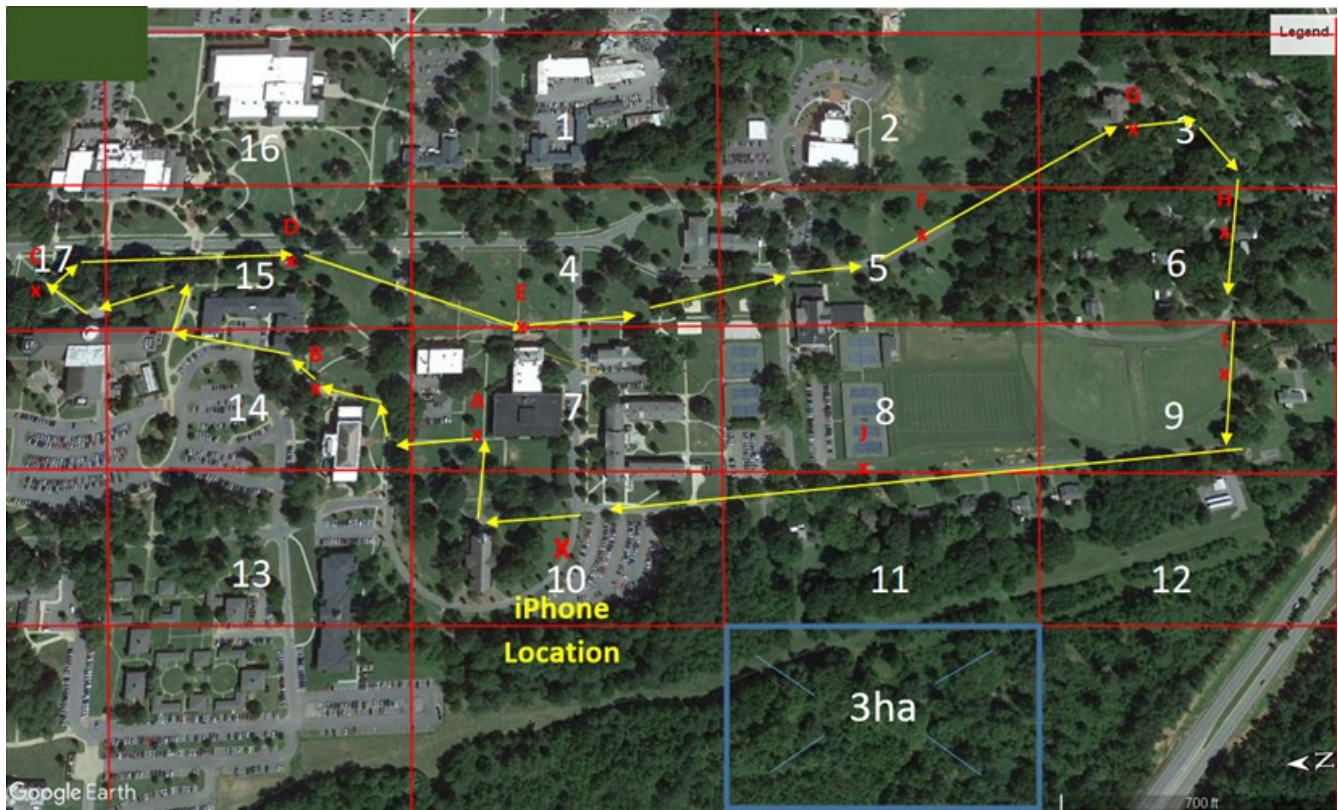
Figure 1. Designated regions (1-17) and specific locations (A-J) to examine Apple Inc. AirTag™ estimated and actual locations (Phase I) and device recovery (Phase II) within a 50-km test area of the Berry College campus, Georgia.
