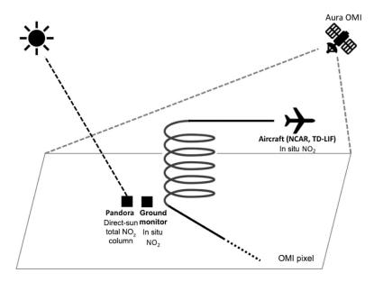
Figure 1. Conceptual illustration of  $NO_2$  observations during the DISCOVER-AQ and KORUS-AQ field campaigns. The instruments used include ground-based monitors measuring in situ  $NO_2$  volume mixing ratios, Pandora making direct-sun measurements to retrieve the total column  $NO_2$ , airborne instruments measuring in situ  $NO_2$  profiles, and the Ozone Monitoring Instrument (OMI) aboard the Aura spacecraft reporting total column and tropospheric column  $NO_2$ .
