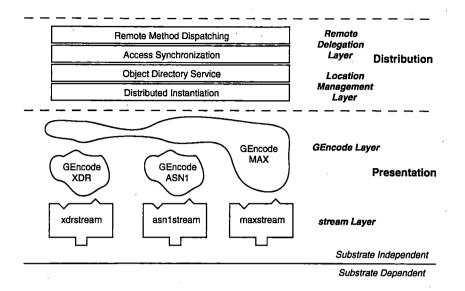
Figure 3: Communication Substrate Independent Level
