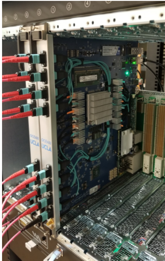
Figure 5.12: Picture of the assembled OCEAN Blade board that will be implemented into the CMS detector hardware. The onboard FPGA will allow for the TPS algorithm to be implemented directly as firmware into the muon trigger in the detector.
