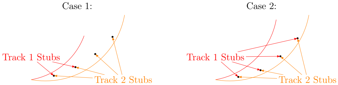
Figure 5.8: Illustration of the two different cases that are considered when cleaning candidate tracks that share detection stubs. In case 1 there are two tracks that share stubs but one track has more stubs than the other. In case 2, the tracks share the same number of stubs, but one track has a smaller sum of the deviation in the propagated \phi values as given in equation 5.12.
