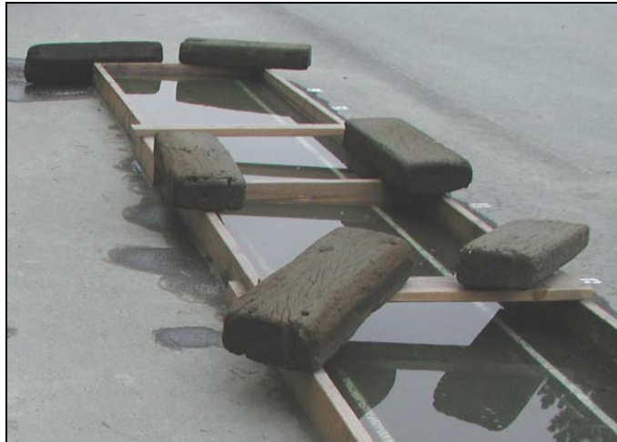
Figure 3.5: Soaking dam with water.
