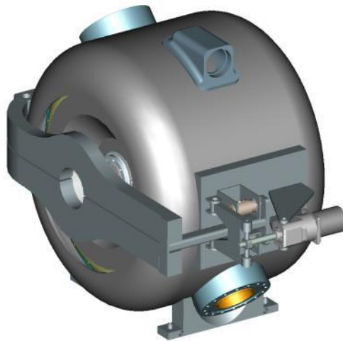
Figure IV-20: SSR1 cavity, helium vessel, and tuner
