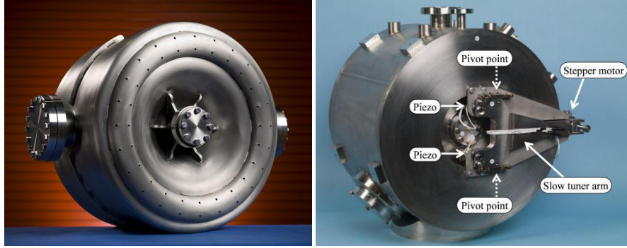
Figure IV-16: Photographs of the bare and dressed prototype SSR1 cavity
