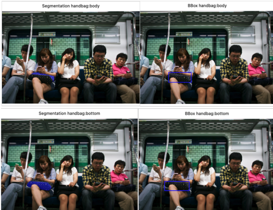
Figure 2.1: (Top) Segmentation-mask and bbox for part-body of object-handbag (bottom) Segmentation-mask and bbox for part-bottom of object-bottom. While the segmentation mask for body and bottom have clear distinctions, the bbox for these parts are overlapping. Sample and annotations taken from PACO dataset.
