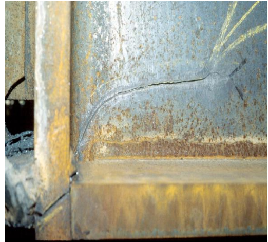
Figure 5-1: Welded Beam-Column Connection Fractures after 1994 Northridge Earthquake (Kanvinde lecture, 2015)
