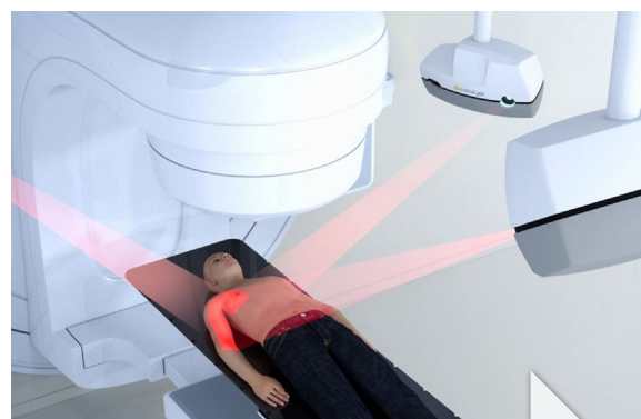
Figure 2 Computer rendering of the Catalyst surface imaging system using ceiling-mounted light source and camera pods. The Catalyst system can project regions-of-interest onto the patient's surface to assist with setup. ( http://c-rad.se/product/catalyst-2/ ). (Color version of figure is available online.)
