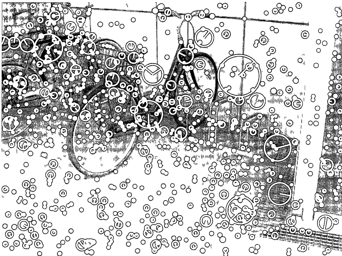
Figure 12 SIFT Detections A sample image from the bike category of the Graz-02 dataset and its detected SIFT features The scale of each feature is the radius of the circle, and the orientation of the feature is denoted by a line through its center
