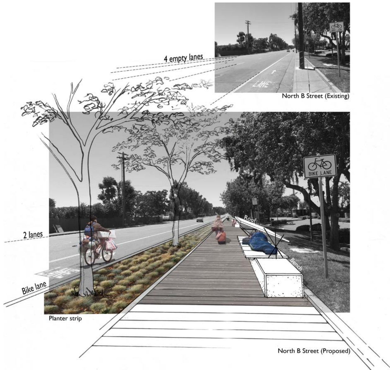
Figure 8.1 N B Street looking west showing existing conditions, as well as potential narrowing of the road and a tree-lined buffer
