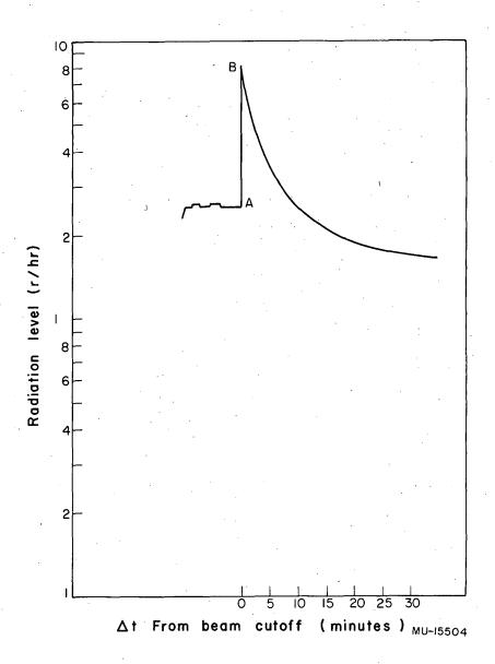
Fig. 4. Typical radiation decay on Speedomax chart. Deuteron particles on Be; 70 µa on target; 3.4 hr bombardment; after 8 hr 0.400 R. A=beam off 1,000 R full scale B=scale change 10 R full scale
