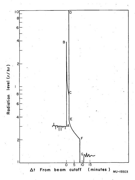
Fig. 3. Typical radiation decay on Speedomax chart.
