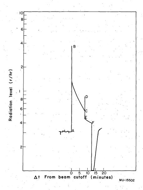
Fig. 2. Typical radiation decay on Speedomax chart.
