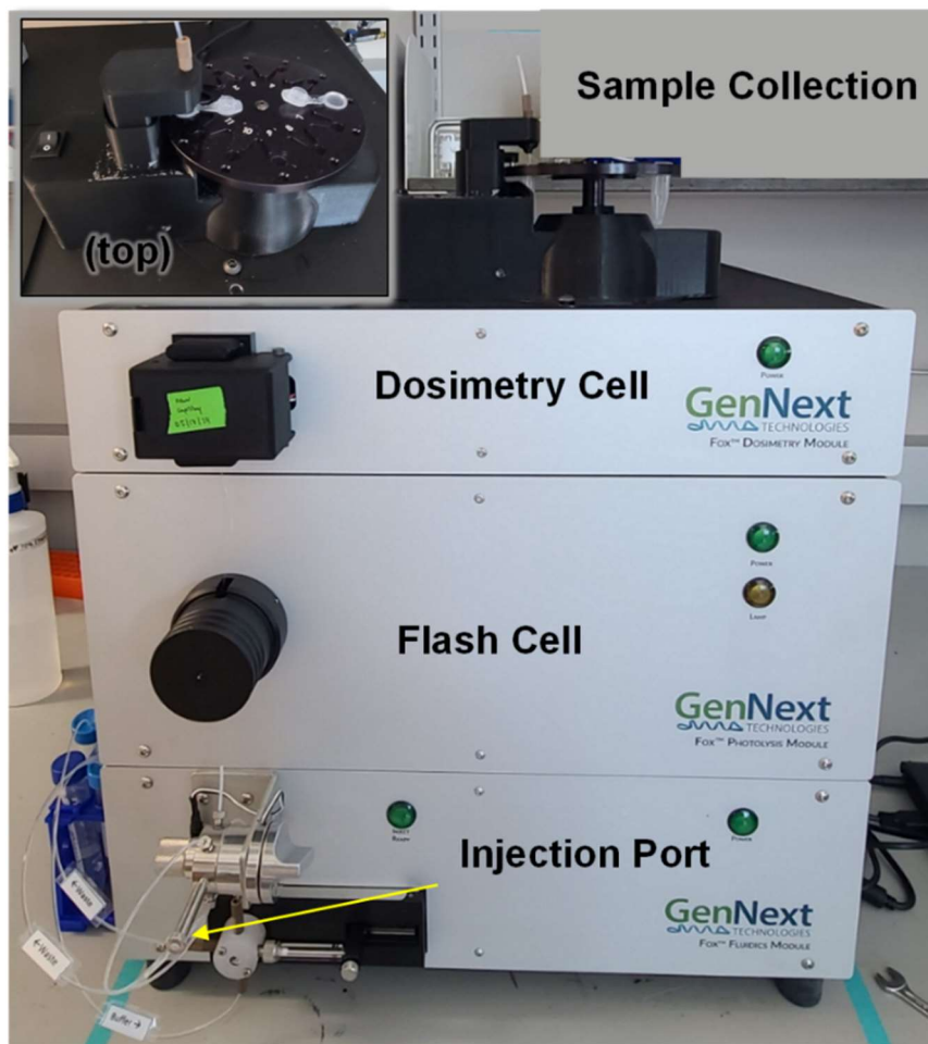
Figure 3. GenNext ® Technologies' semi-automatic FOX ® system. Sample is injected at the fluidics module, irradiated at the photolysis module, and collected after dosimeter absorbance is measured at the dosimetry module.
