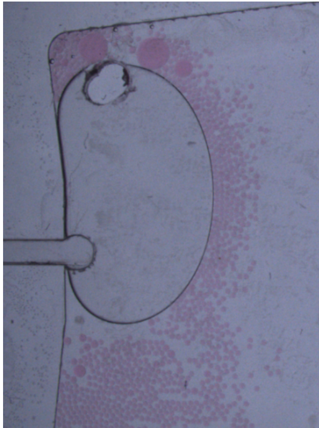
Figure 4.4: Droplets from dilute agarose solution
