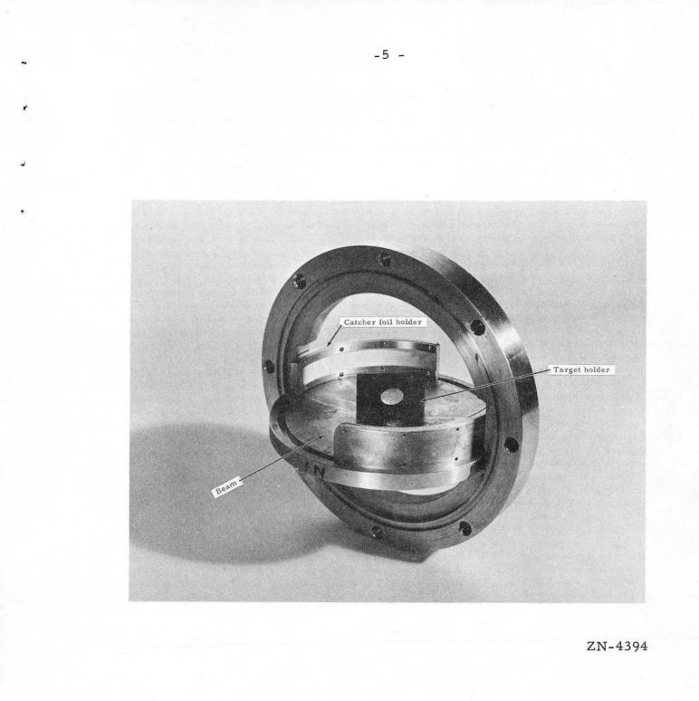
Fig. 2. Angular distribution apparatus. This angular distribution apparatus is capable of determining the laboratory angular distribution of recoils at all angles.
