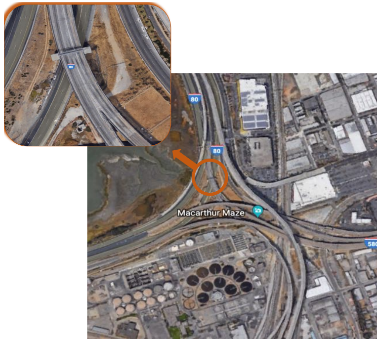
Figure 1.1: Satellite imagery from Google Earth of the MacArthur Maze with an enlarged view of a typical diverge with a bifurcating lane.
