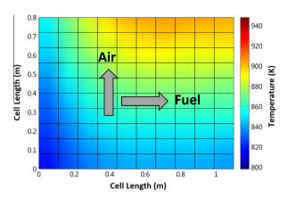
Fig. 2. Steady-state electrolyte temperature profile generated using the current spatially resolved dynamic fuel cell model.
