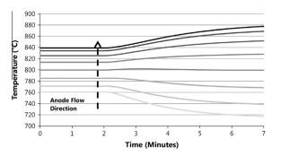
Fig. 8. Spatial temperature response of a simulated 1 MW Oxy-FC to a rapid load increase.
