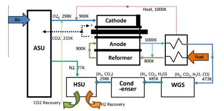
Fig. 1. Poly-generating Oxy-FC system configuration concept and integration schematic.
