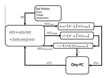
Fig. 5. Oxy-FC part-load and thermal management controller.
