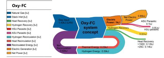
Fig. 3. Sankey diagram of energy flows for the Oxy-FC concept at 10 atm and 750 mW cm<sup>-2</sup>.
