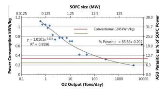
**Fig. 4.** Summary of ASU performance and parasitic load that it would require from the Oxy-FC system design.
