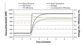
Fig. 7. Simulated Oxy-FC transient response to a rapid load increase from 50% to 100% load for a 1 MW system.
