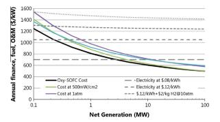
Fig. 9. Annual Oxy-FC cost compared with grid baseline with hydrogen recovery potential.
