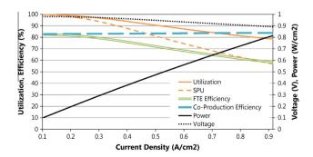
Fig. 6. Part load fuel cell operating conditions and performance characteristics.
