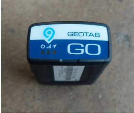
Figure 3-4. Geotab GO monitoring device
