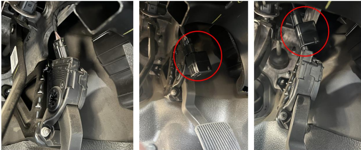
Figure 3-6. A) Electronic accelerator pedal without SmartPedal™ installed, B) SmartPedal™ connected to accelerator pedal wire harness connection, C) SmartPedal™ installed inline between accelerator pedal and accelerator pedal wire harness connection.
