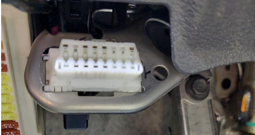
Figure 3-2. 16-pin J1962 OBD II port
