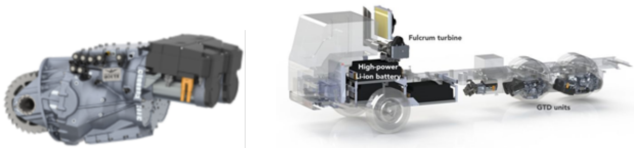
Figure 26. Wrightspeed powertrains, with fulcrum turbine (right) SOURCE: Wrightspeed Presentation, “Powertrains - Scaling up,” CEC, CEC Fuels and Transportation Merit Review, December 2, 2015
