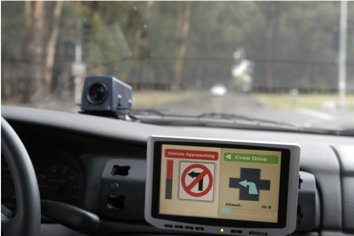
Figure 4-4. DVI mounted in the Taurus displaying the No-Left-Turn Warning.
