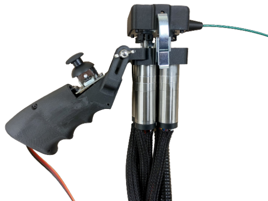
Figure 2.11: This is a recent revision using Maxon EC motors.
