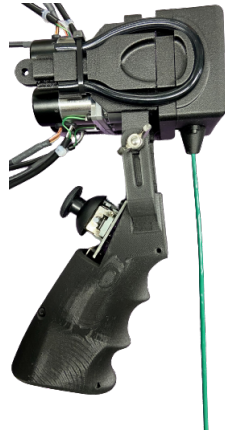
Figure 2.7: Above is an early revision of the motor housing that used a rubber strip to contain the various motor housing parts together.
