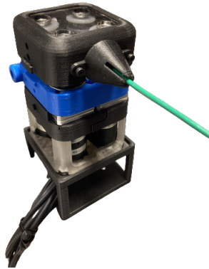
Figure 2.9: Above is the current revision of the handheld base without clamp that features the disposable top, motors, and motor housing on an upright, removable base.
