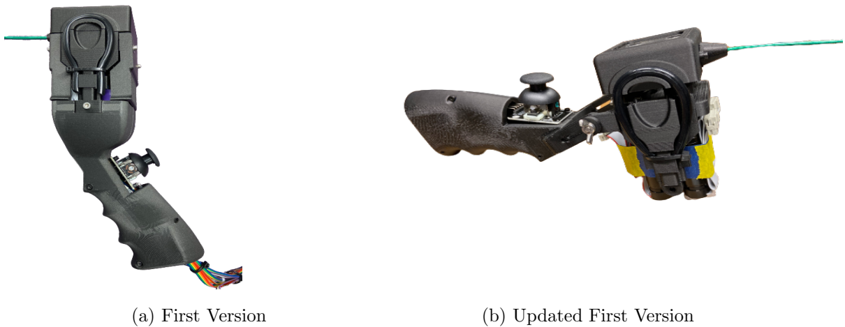
Figure 2.3: (a) First motor housing revision with Maxon DC motors using a rubber strip to contain the various motor housing parts together, and (b) an early revision with an updated handle and motor housing design using the same Maxon DC motors.
