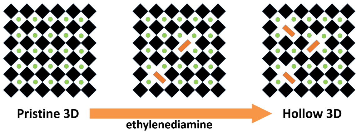
Figure 5. Schematic illustration of the structure of the 3D pristine \text{MAPbI}_3 perovskite and its transformation from a dense proper perovskite structure to a hollow 3D structure with increasing amount of en . Black cubes: [\text{PbI}_6] octahedra, green spheres: MA cations, orange rectangles: ethylenediammonium ( en ) cations.
