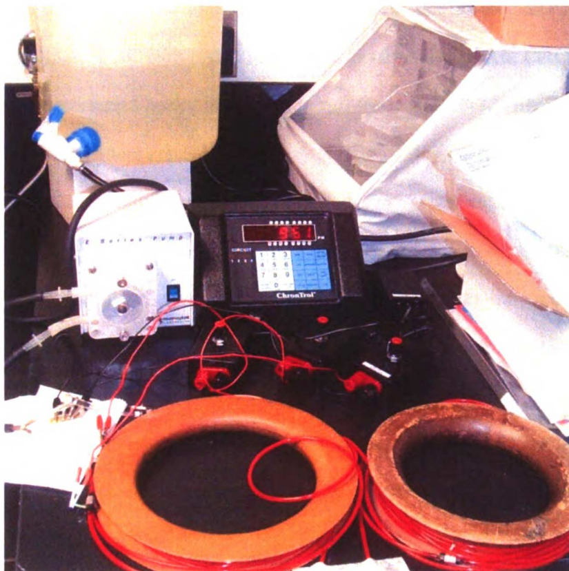
Figure 1: The experimental setup including the coil of test DUWL on the left side and the control DUWL on the right side. Behind the coils are the current controllers, the peristaltic pump and electronic timer, and the 10L carboy reservoir.
