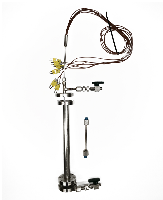
Figure 5.S6. Photograph of large-scale (1" OD pipe, 12" long) and small-scale (1/4" OD pipe, 6" long) breakthrough columns used in this work.
