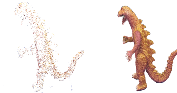
Figure 5.1: An initial sparse reconstruction, with good camera estimation, on the left. It can be made into a very dense version, on the right, by our method.
