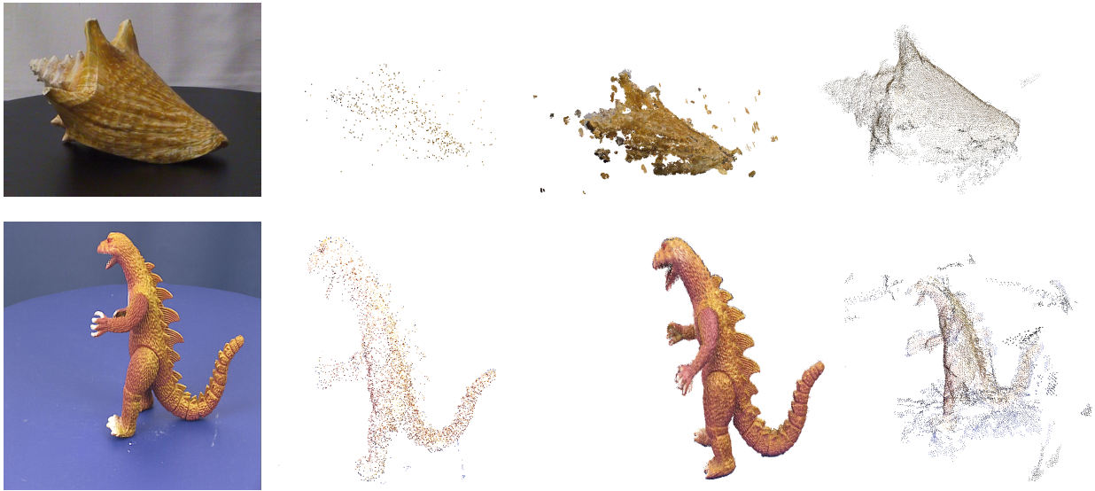
Figure 5.5: Results from the proposed method for the Dinosaur and Conch datasets. The first column shows an example input image, the second shows the initial sparse reconstruction used as input, the third shows results from the proposed method, and the last column shows the result of CMVS/PMVS as implemented by VisualSfM. For the Conch shell dataset with 216 images of size 640x480, our method takes 3 minutes. For the Dinosaur dataset with 36 images of size 720x576, our method takes 1.3 minutes.
