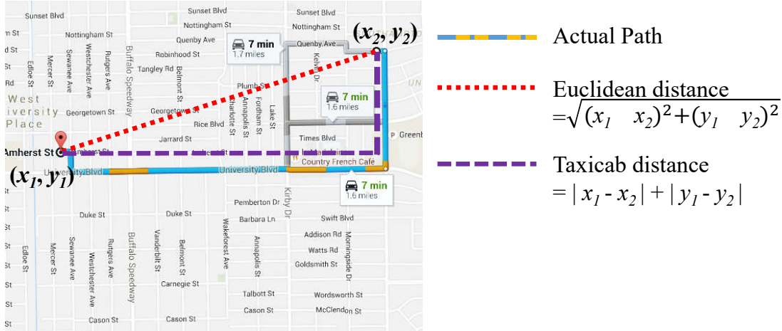
Figure 6.9. Illustration of the actual path, Euclidean distance and taxicab distance
