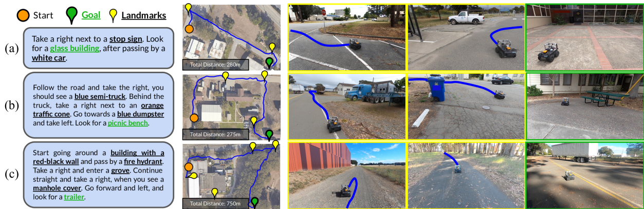
Figure 52: Qualitative examples of LM-Nav in real-world environments executing textual instructions (left). The landmarks extracted by LLM (highlighted in text) are grounded into visual observations by VLM (center; overhead image not available to the robot). The resulting walk of the graph is executed by VNM (right).
