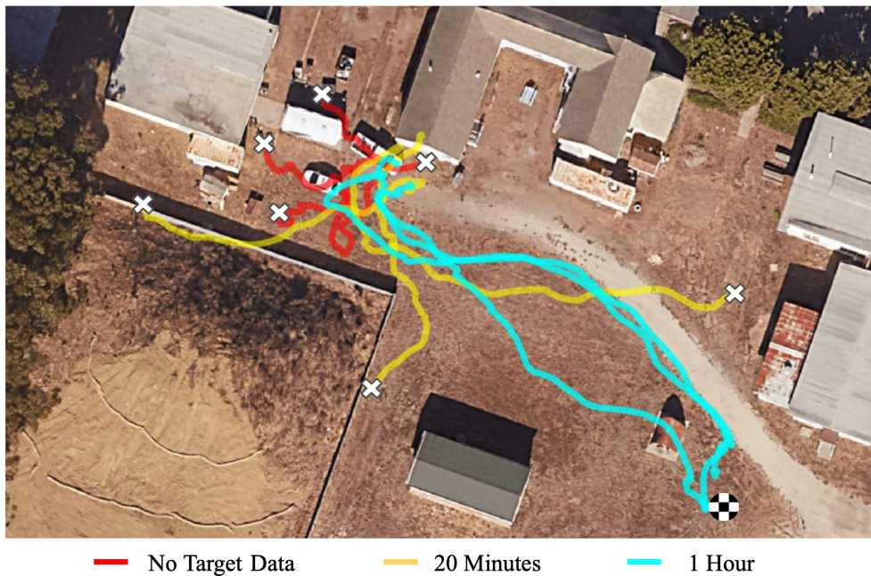
Figure 6: Fast Adaptation to a New Environment: After training ViNG in one environment, we deploy the system in a novel environment, shown above. By practicing to reach self-proposed goals and using that experience to finetune the controller, ViNG is able to quickly gain competence at reaching distance goals in this new environment, using just 60 minutes of experience. Example rollouts towards a goal 35m away (marked by checkerboard circle) demonstrate ViNG self-improving from interactions in the barracks environment.
