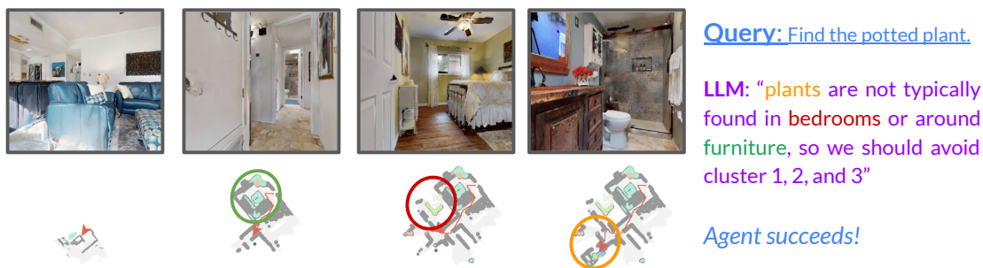
Figure 58: Qualitative example of a negative score influencing the agent’s decision. LFG discourages the agent from exploring the bedroom and living room, leading to fast convergence toward the goal, whereas FBE fails. The CoT reasoning given by the LLM is shown in purple, justifying its score.
