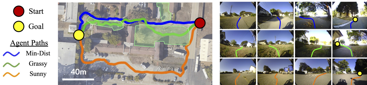
Figure 26: Comparison of policies for different reward functions learned by ReViND. Left: an overhead map (not available to the method), with grassy areas indicated with green shading. Note that the policy for the “sunny” reward chooses a significantly different path through a concrete parking lot without tree cover, while the policy for the “grassy” reward takes frequent detours to drive on lawns. Right: first person images during each traversal, with the chosen path indicated with colored lines.
