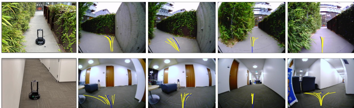
Figure 47: Visualizing rollouts of NoMaD deployed in challenging indoor (top) and outdoor (bottom) environments on the LoCoBot platform, showcasing successful exploration trajectories. Future action samples from the undirected mode are shown in yellow, and the action selected by the high-level planner is shown in blue. The predicted actions follow implicit navigational affordances, such as following hallways, and become multimodal at decision points, such as intersections in the hallway.
