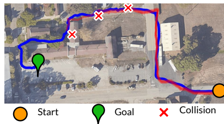
Figure 54: GPS-Nav (red) fails due to its inability to reason about traversability through obstacles, while LM-Nav (blue) succeeds.
