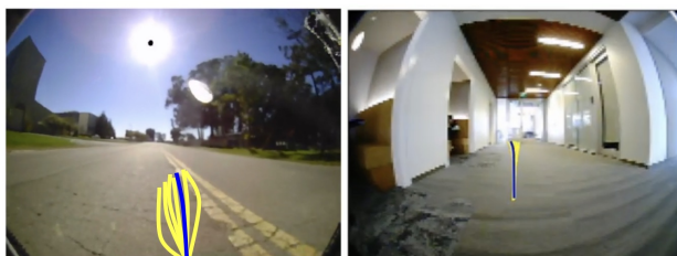
Figure 42: ViNT exhibits an implicit preference for following paved roads ( left ) and hallways ( right ).
