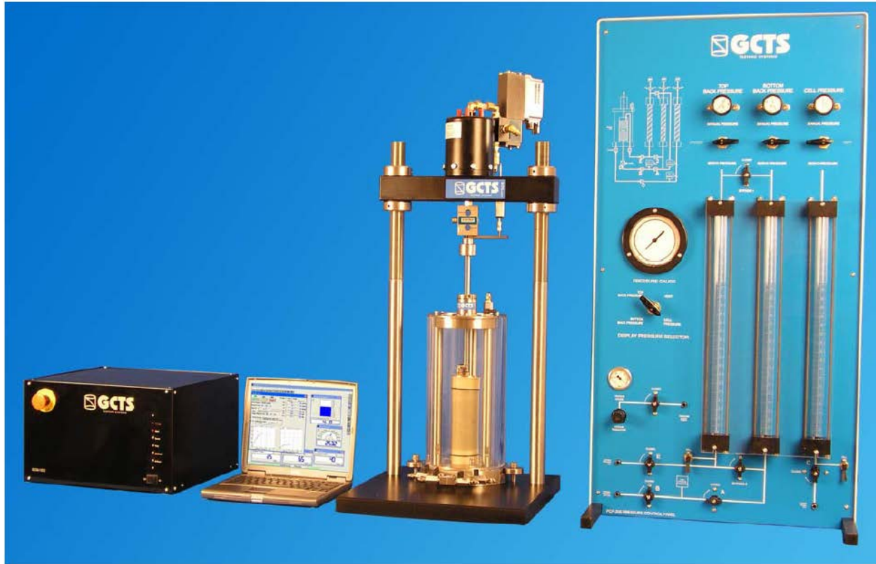
Figure 3.5. GCTS STX-050 electro-pneumatic cyclic triaxial device with PCP-200 pressure control panel
