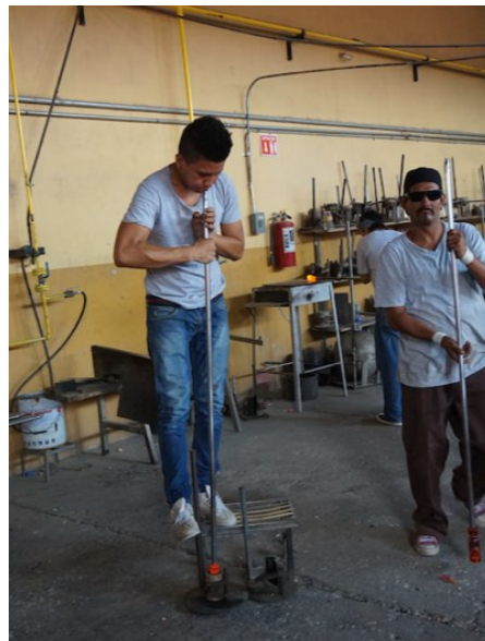
Figure 88. Glassmaker in Jalisco using a dip-mold to make a shot glass (photo: Karime Castillo).
