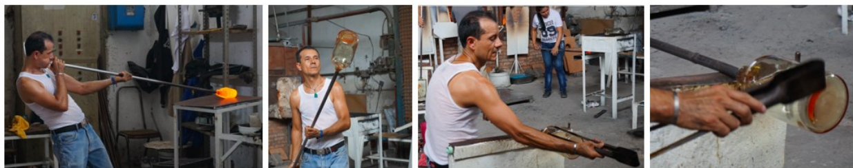
Figure 79. Glassblower in Jalisco making a free-blown bottle (photos: Karime Castillo).
