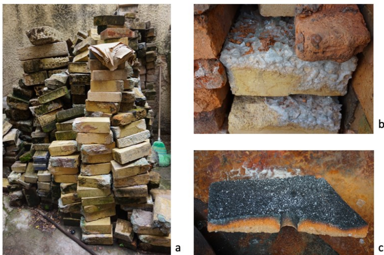
Figure 73. Waste from modern furnaces in Jalisco, Mexico: a) pile of bricks from a dismantled furnace; b) tank furnace bricks with remain of glass; c) fragment of a gathering hole cover showing deterioration on the side exposed to the heat (photos: Karime Castillo).
