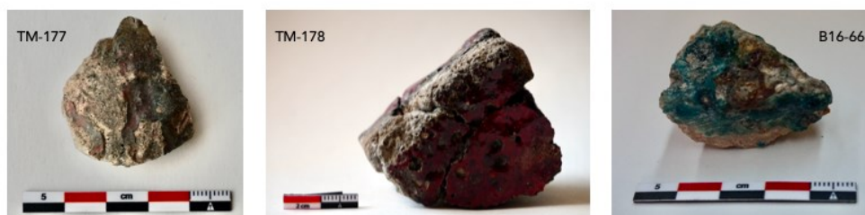
Figure 76. Fragments of crucibles with red and blue-green glass (photos: Karime Castillo).
