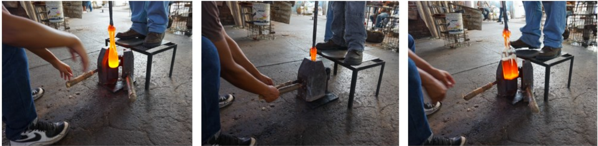
Figure 91. Artisans in Jalisco making a bottle using a two piece mold (photo: Karime Castillo).
