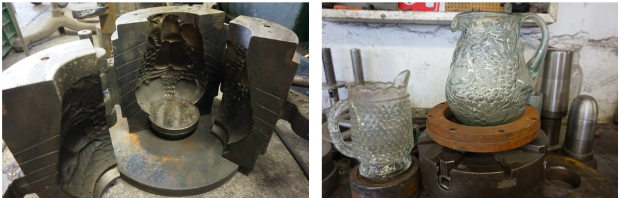
Figure 95. Mold for making a pressed glass vase with elaborate decoration (left) and two finished pressed glass objects, a cup and a jug (right) (photos: Karime Castillo).
