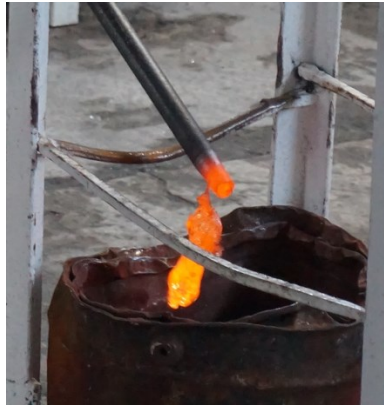
Figure 68. Disposal of excess glass (photo: Karime Castillo).
