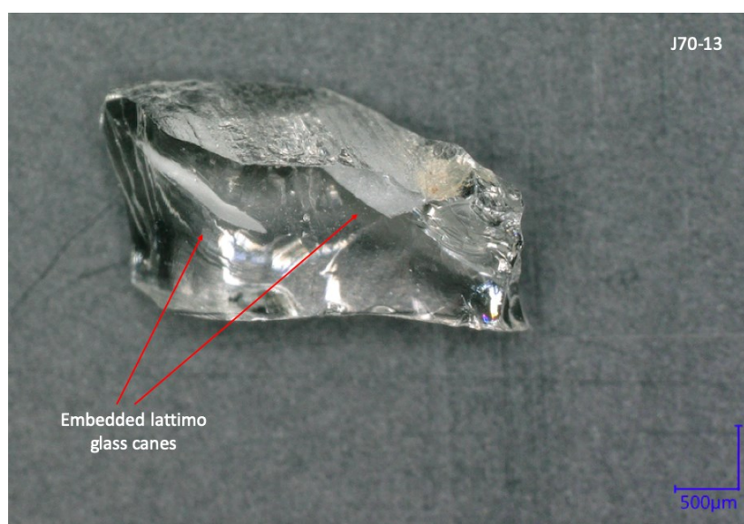
Figure 152. Sample of Venetian glass fragment with embedded lattimo canes (magnification: 50x).
