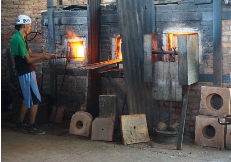
Figure 55. Ceramic “doors” or covers at the feet of a glass furnace in Jalisco (photo: Karime Castillo).
