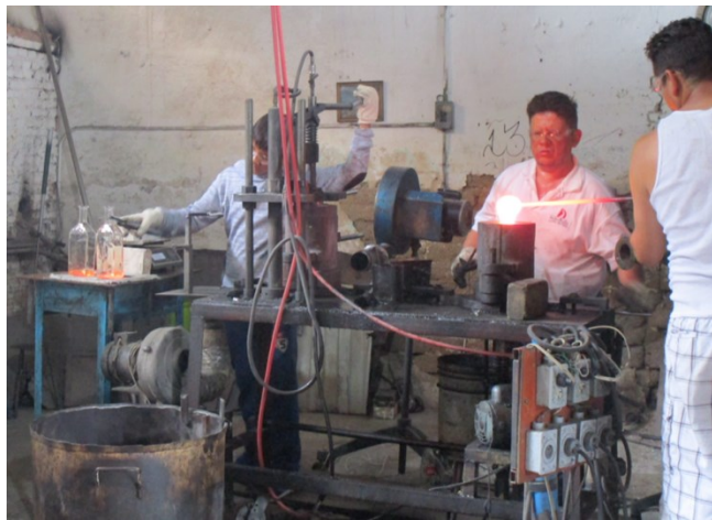
Figure 98. Glass artisans in Jalisco operating a semi-automatic bottle-making machine.
