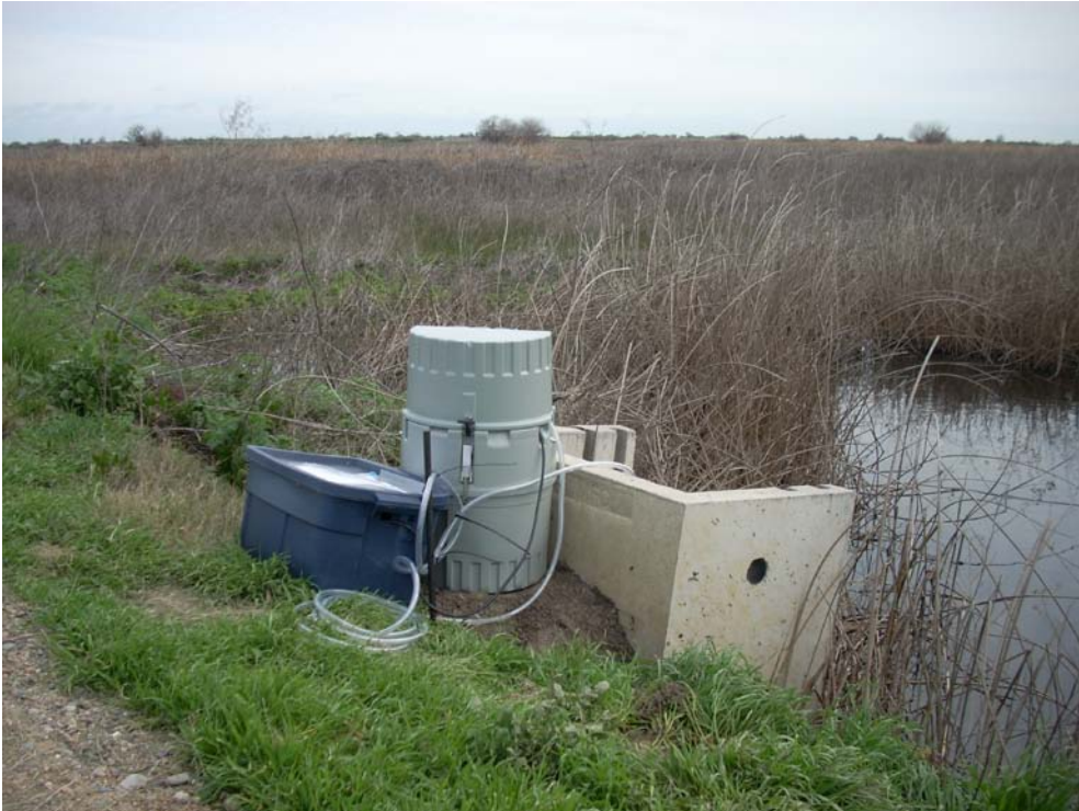
Figure 3-17: Los Banos Wildlife Management Area pond 38 drainage site showing deployment of an auto-sampler.
